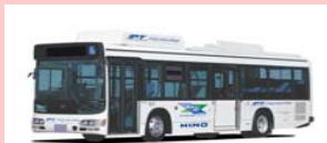
IPS ( non-contact recharging ) hybrid bus
